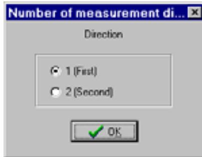
Select one of the two measurement directions for balance and correction weight calculation and press the **OK** button.
