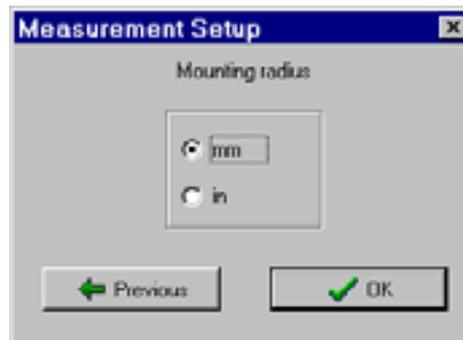
After you selected metric (mm) or English units for mounting radius, the Calculation of Residual Unbalance dialog will be displayed to enter mounting radius for each balance plane in use.
