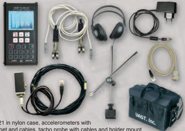
DC-21 in nylon case, accelerometers with magnet and cables, tachometer probe with cables and holder mount with magnet, charger, communication cable, headphones. The DC-21 kit is supplied in a nylon bag. Vibro12 application software is included in the kit.
